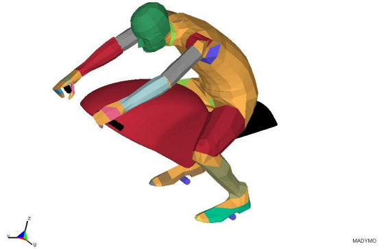
Madymo model representing a human facet model and the human-motorcycle interface geometry
